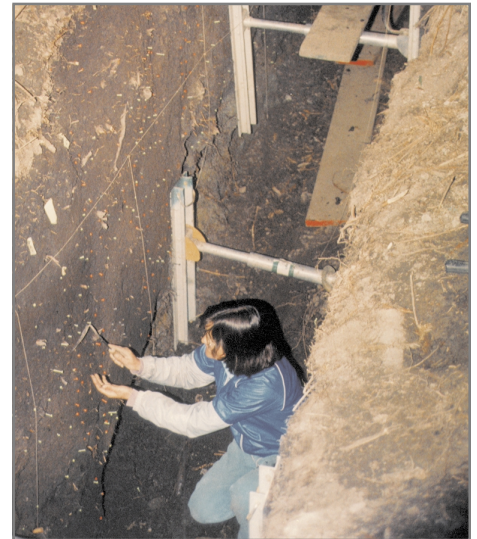
In this deep trench dug across the San Andreas Fault near Loma Prieta peak, California, U.S. Geological Survey scientists identified soil layers disrupted by the last great earthquake before the 1906 San Francisco earthquake (magnitude 7.8). Radiocarbon dating of plant remains from the layers in the trench indicates that the earlier quake occurred about A.D. 1600, before written historical records were kept in California.
